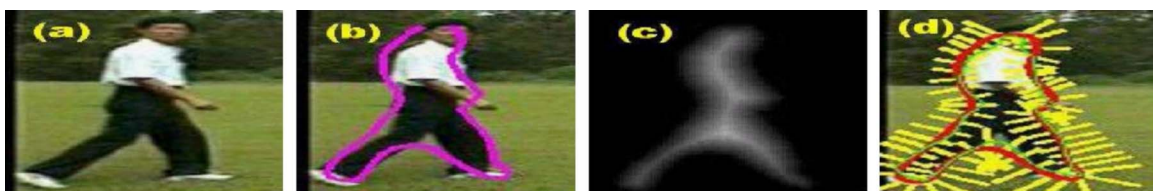
Fig. 3. (Color online) Example of how to make a normal line scanning adaptive. (a) Cropped original object, (b) estimated contour, (c) the distance transformed object, (d) normal lines on control points.
