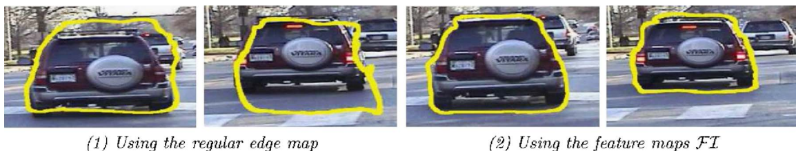
Fig. 5. (Color online) Performance comparisons on a cluttered scene. A stabilization step is applied to obtain the second set of results to obtain FI because the sequence was acquired by a moving camera.
